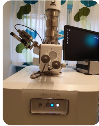
Figure 11. Characterization of microstructure and chemical composition, a) optical microscope, b) Scanning Electron Microscope (SEM).
