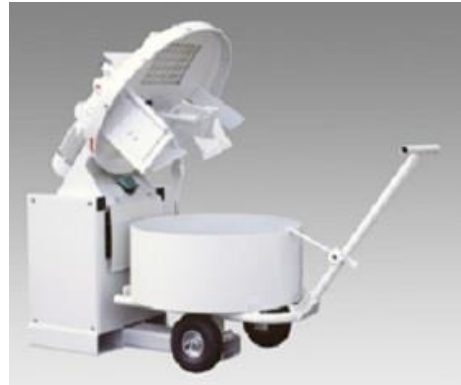
Figure 7. Mixing equipment, a) 8 – litter “Hobart” mixer, b) Zyklos pan mixer.
