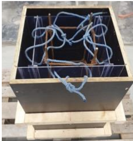
Figure 10 Formwork preparation before casting with reinforcement and moving plates installed.
